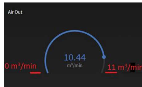
Figure 71 - relation of the member group settings to the range of the gauge
