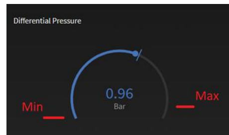
Figure 63 - Gauge and related setting of the range as appearing on local AERO dashboard
