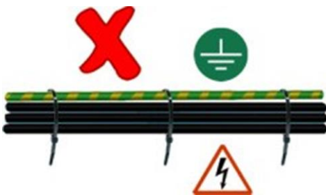
Figure 13 - How not to place cables part 2
