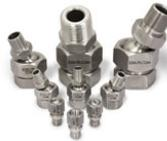
EXAIR's Swivel Fittings make it easy to adjust the position of the Air Nozzles, Air Jets, and Air Amplifiers. Swivel Fittings permit a movement of 25 degrees from the center axis for a total movement of 50 degrees. Type 303 and 316 stainless steel.
