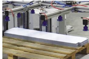
A series of bellows cups lift one plastic part at a time off a pallet.
