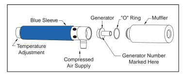
To change generators (white plastic part), firmly grip the blue sleeve while unscrewing the muffler (counterclockwise). Note the position of the "O"-ring and generator during disassembly. Install the desired generator. (The flow rate is stamped on each generator.) Lower capacities produce less refrigeration and cold flow with reduced compressed air consumption.
