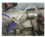
The Adjustable Spot Cooler maintains critical tolerances on machined plastic parts.
