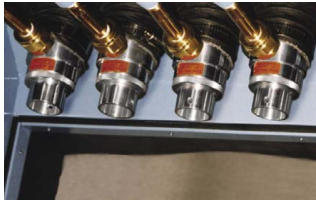
Adjustable Air Amplifiers are ducted to draw clean air for drying.
