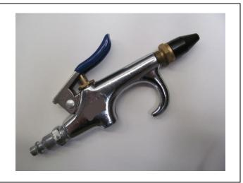
**BEFORE EXAIR:** This customer had used a third party to perform a safety audit in their facility. It was found that the production area sound level was on average over 93 dBA. This was far exceeding the OSHA allowable noise level for no hearing protection. The existing blowoff gun also failed to meet or exceed OSHA's dead end pressure standard CFR 1910.242(b). The noise level in the area needed to be lower than 84 dBA, on average.
