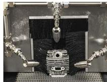
A combination of Model 6013 High Velocity Air Jets dry this chainsaw cylinder head.
