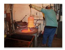
**BEFORE EXAIR:** Customer was using (3) 24" (610mm) industrial shop fans to cool the tooling piece from 1,725°F to less than 600°F. The engineer's intent was to provide a turntable system to rotate the part, while blowing it with a greater volume of air, to effect faster cooling. The fans needed <u>almost a half an hour to cool the part to 600°F</u>, and their goal was to reduce this to 20 minutes or less.
