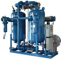
Heated blower purge, activated alumina desiccant dryer with Energy Management System (EMS) and 2% purge rate
