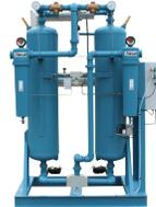
Externally heated desiccant dryer with mid-bed energy management based on relative humidity and a purge flow rate of 8% (6% with venturi option)
