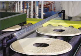
Model 110054 54" (1372mm) Super Air Knife dries stamped parts that exit a washer.
