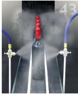
(2) Model EB1040SS nozzles are used to rinse wine bottles after capping.
