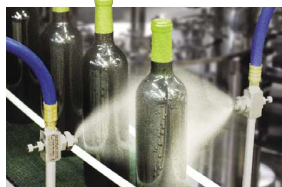
(2) Model EB1030SS atomizing nozzles are used to give a final sanitary rinse prior to labeling wine bottles.
