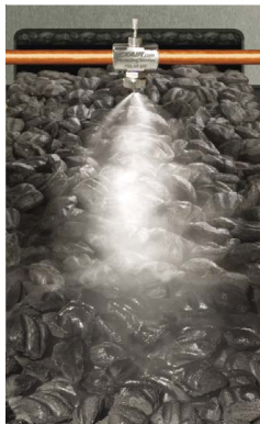
A Model AW1030SS is used to keep dust down during charcoal briquette production.
