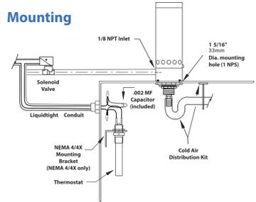
The Cabinet Cooler mounts to the enclosure through a drilled hole or electrical knockout. The NEMA 12 (IP54) Cabinet Coolers may be mounted on the top or side of the panel. NEMA 4 and 4X (IP66) Cabinet Coolers must be mounted on the top of the panel or on the side of the panel using one of our Side Mount Kits (See page 198).
