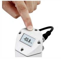
Alarm adjustment at dew point sensor
