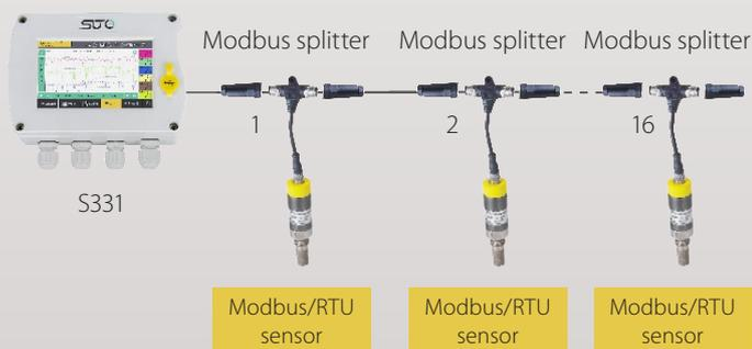
The Modbus/RTU bus allows to connect several sensors to a single bus line via Daisy-Chain.
