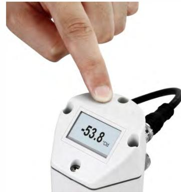
Alarm adjustment at dew point sensor
