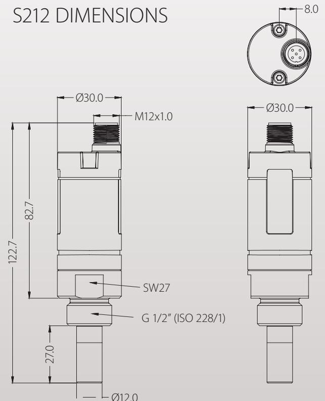
The SUTO dew point sensor S212 provides reliable and long term stable dew point monitoring in industrial applications. The newly developed sensor features improved signal and stability in demanding industrial applications. It makes it an ideal choice for dew point measurements in desiccant dryers.
