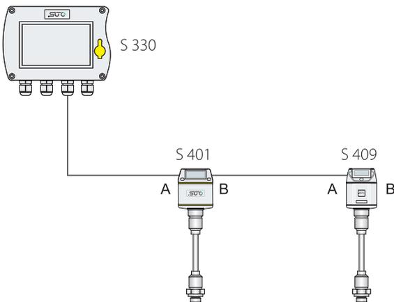
**Attention:** Flow sensors S 450/S 401 need to have the bi-directional calibration option to operate in both directions
