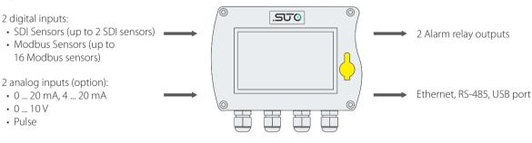
SUTO sensors are equipped with SDI and / or Modbus interface
