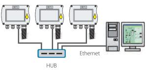
S4M acquiring measurement data through Ethernet from several remote units
