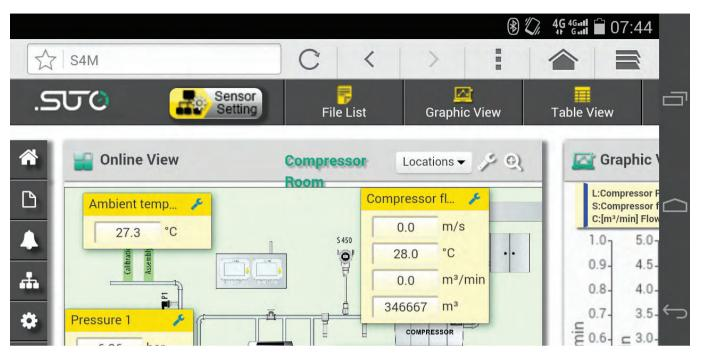
Above is an example show monitoring of a typical compressed air system with all relevant online parameters displayed on the screen.
