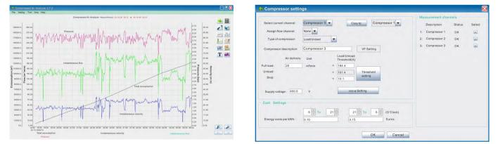
Through SUTO software S4A recordings are downloaded to the PC via USB or Ethernet port. The basic analysis can be done in S4A.
