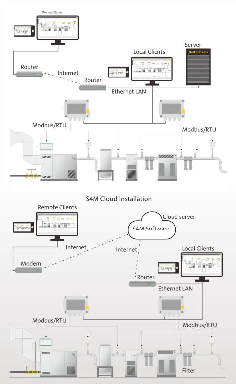
S4M helps you to keep your plant under your control. Gathering the date of all installed sensors and measurement system. Combining them into a single software solution which enables you to take back the control of your system.
