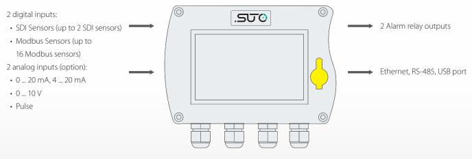
SUTO sensors are equipped with SDI and / or Modbus interface
