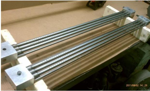
**BEFORE EXAIR:** The customer is running a homemade drilled pipe configuration to help cool and set the surface layer of hot extruded polymer sheet. Notice in the picture below you can see the streaks the holes in the pipe are causing to the surface finish.
