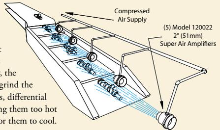
**The Solution:** They installed (5) **Model 120022 2" (51mm) Super Air Amplifiers** over the shake-out conveyor. The high output airflow from each Super Air Amplifier rapidly cooled the parts without shocking them (no cracks or imperfections from cooling too rapidly). **When the part reached the end of the conveyor, the operator could proceed immediately.** The backlog was completely eliminated.
