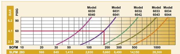
Total Output Flow with .002” (0.05mm) gap setting. Excludes downstream entrainment.
