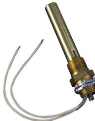
The adjustable thermostat is factory set at 95°F (35°C). It will normally hold ±2°F (1°C) of the desired temperature setting. It is rated 24V-240V AC or DC, 50/60Hz and is UL Recognized, CSA Certified.
