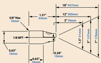
The Model HP1136SS Shim Set for the 1" High Power Flat Super Air Nozzle includes a .020" (0.51mm) and .030" (0.76mm) thick shim. A .025" (0.64mm) shim is installed.
