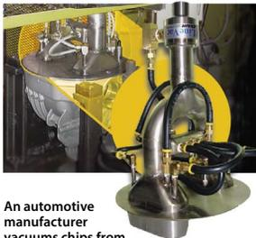
An automotive manufacturer vacuums chips from drive train differentials with a Model 150200 2" (51mm) Heavy Duty Line Vac.
