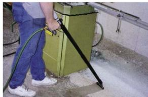
**Model 6192 Vac-u-Gun Collection System with bag vacuums absorbent and chips.**
