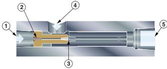
Compressed air flows through the inlet (1), then through a single directed nozzle (2). As the airstream exhausts, it expands and increases in velocity prior to passing through the venturi (3). A vacuum inlet tangential to the primary airflow (4) is located at the suction point between the orifice and the venturi. The airflow that is drawn through the vacuum inlet mixes with the primary airstream, then exhausts on the opposite end (5).
