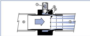
Compressed air flows through the inlet (1) into an annular plenum chamber (2). It is then injected into the throat through directed nozzles (3). These jets of air create a vacuum at the intake (4) which draws material in and accelerates it through the unit (5) for conveying over long vertical or horizontal distances.
