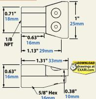
The 1" and 2" Flat Super Air Nozzles are shipped with a .015" (0.38mm) air gap opening that is set with a stainless steel shim positioned between the cap and the body. Force and flow may be easily increased or decreased by installing a different shim.
