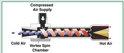
The Mini Cooler incorporates a vortex tube to convert a small amount of compressed air into two low pressure streams, one moving within the other in opposite directions (see page 173). The two airstreams exchange heat, producing cold air from one end of the tube and hot air from the other. A flexible hose directs the cold airstream at the surface to be cooled.
