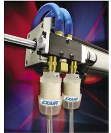
Each Reclassifying Muffler passes a certain volume of air with minimal back pressure restriction so it doesn't interfere with the operation of the cylinder or valve. When used with cylinders, the "Muffler Quick Pick" table (*right*) helps you select the appropriate model based on the actual bore and stroke of the cylinder.
