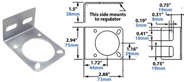
This optional mounting bracket fits Models 9008, 9033 and 9009 Pressure Regulators and includes a locking ring.
