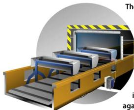
The timer was set to "interval" and the sensor mounted next to the Super Ion Air Knives. When it detected a bumper, it immediately turned on the air for 10 seconds. If the conveyor stopped, it would not turn the air on again until it detected the next bumper.
