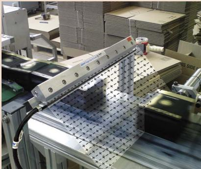
**The Problem:** A manufacturer of perfumes and fragrances had a problem with the packaging of their fine perfumes. The conveyor belt used to transport the boxes to the cellophane sealer rubbed against the box surface and induced a sizable static electricity charge on it that made it a "dust magnet". The cardboard dust and particulates
