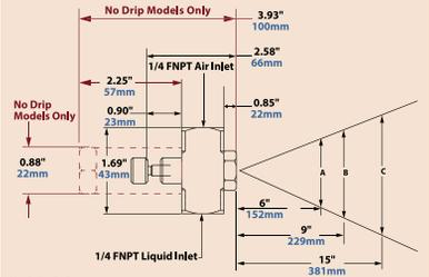
No Drip Only Dimensions in Red See page 90 for No Drip Atomizing Nozzles
