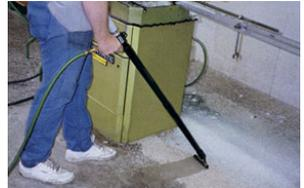
**Model 6192 Vac-u-Gun Collection System** with bag vacuums absorbent and chips.
