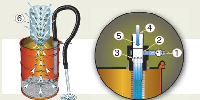
Compressed air, normally 80-100 PSIG (5.5 - 6.9 BAR), flows through the inlet (1) into an annular plenum chamber (2). It is then injected into the throat through directed nozzles (3). These jets of air create a vacuum at the intake (4) which draws material in, accelerates it through the unit (5), and directs it to the bottom of the drum. The airflow exhausts through the port in the drum lid. Airborne particles are trapped by the filter bag (6).
