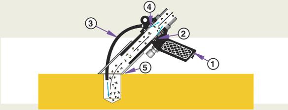
Compressed air, normally 80-100 PSIG (5.5 - 6.9 BAR), flows through the inlet (1) into an annular plenum chamber (2) when the trigger is depressed. A small amount of air is injected into the blow tube (3) to
