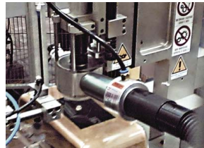
1-1/4" (32mm) Line Vac is mounted on a burr removal tool to suction the plastic shavings and transport them to a waste container.
