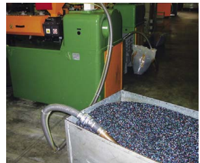
The Model 6083 1-1/2" (38mm) Line Vac conveys plastic granules to the gravity feed hopper on an extruder.
