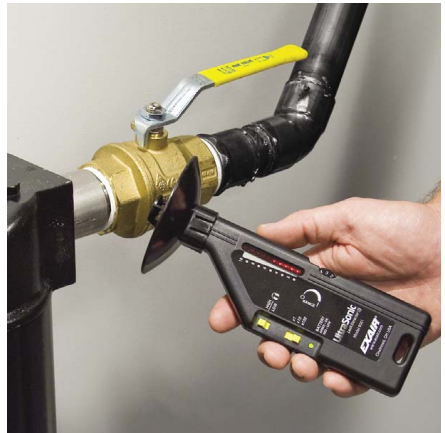
The Model 9061 Ultrasonic Leak Detector quickly pinpoints a costly leak in a noisy industrial environment.
