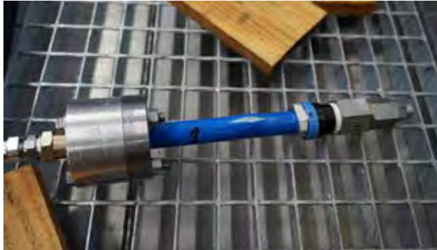
Test at 7700 PSI (535 bar) Pipe bursts but no failure of the fittings.
