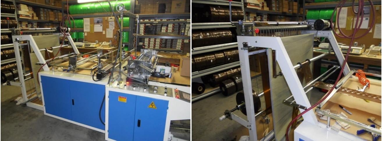
**BEFORE EXAIR:** Before the Super Ion Air Knives were installed, a medical product packager was having issues with the bag material climbing the tension curtain which would cause misfeeds, irregular bag length, material tracking issues and a considerable amount of down time. The machine had a “static eliminator” on it from the factory but that did not seem to work.
