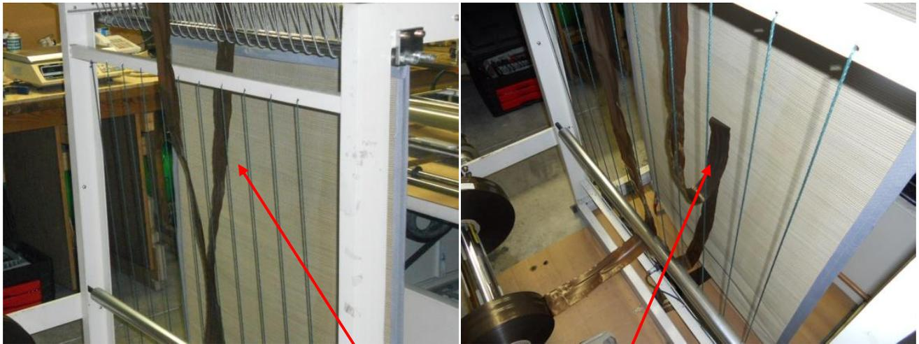
When the tension curtain builds a static charge it makes the bag material cling to the curtain instead of passing under it.
