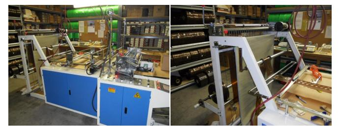
**BEFORE EXAIR:** Before the Super Ion Air Knives were installed, a medical product packager was having issues with the bag material climbing the tension curtain which would cause misfeeds, irregular bag length, material tracking issues and a considerable amount of down time. The machine had a "static eliminator" on it from the factory but that did not seem to work.
