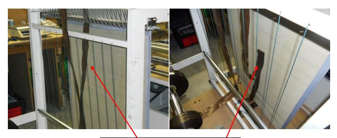
When the tension curtain builds a static charge it makes the bag material cling to the curtain instead of passing under it.
