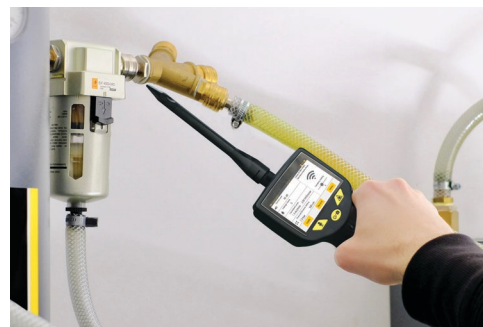
Leak detection with focus tube
