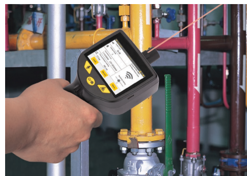
Leak detection from distance with the integrated laser pointer
