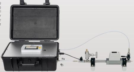
S600 with the isokinetic sampler attached
