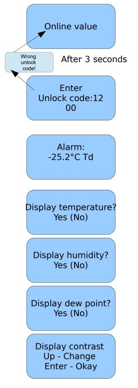
1. At first keep the Enter key ( ⊕ ) pressed for three seconds. Then the S201 will ask to enter the unlock key.
