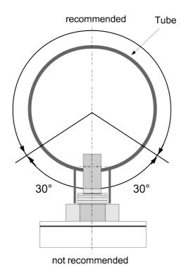
Please install the sensor only in the recommended area like you can see in the picture. A upside down installation is not permitted. Please consider that the distance to the vertical level must be  $>30^{\circ}$ .
