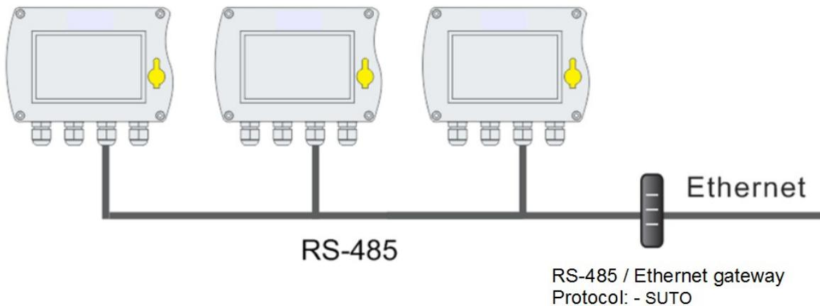
In areas where Ethernet is not accessible, RS-485 can be used to wire the instruments to an access point for Ethernet. Through the RS-485 / Ethernet gateway the link to Ethernet is established. The gateway can handle up to 30 S330/S331. Please ensure that SUTO Bus protocol is selected on S330/S331 menu and every S330RS-485 / Ethernet gateway
