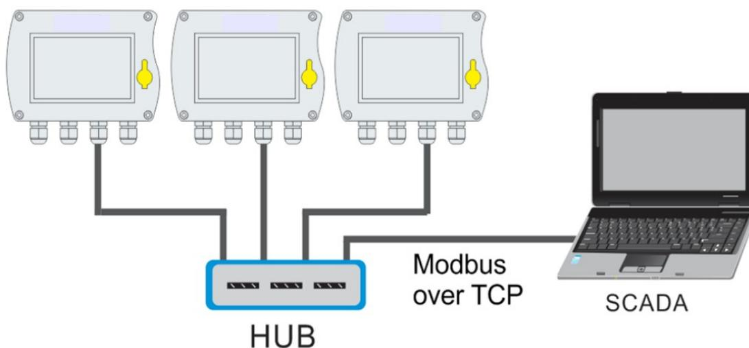
S330/S331 comes with an Ethernet interface. By selecting the Field-bus Ethernet protocol from the S330/S331 menu, the communication with a Modbus master can be established. This is a popular way to connect to a Modbus Master through Ethernet. Process visualization systems are using so-called OPC servers to establish the link to Modbus.
