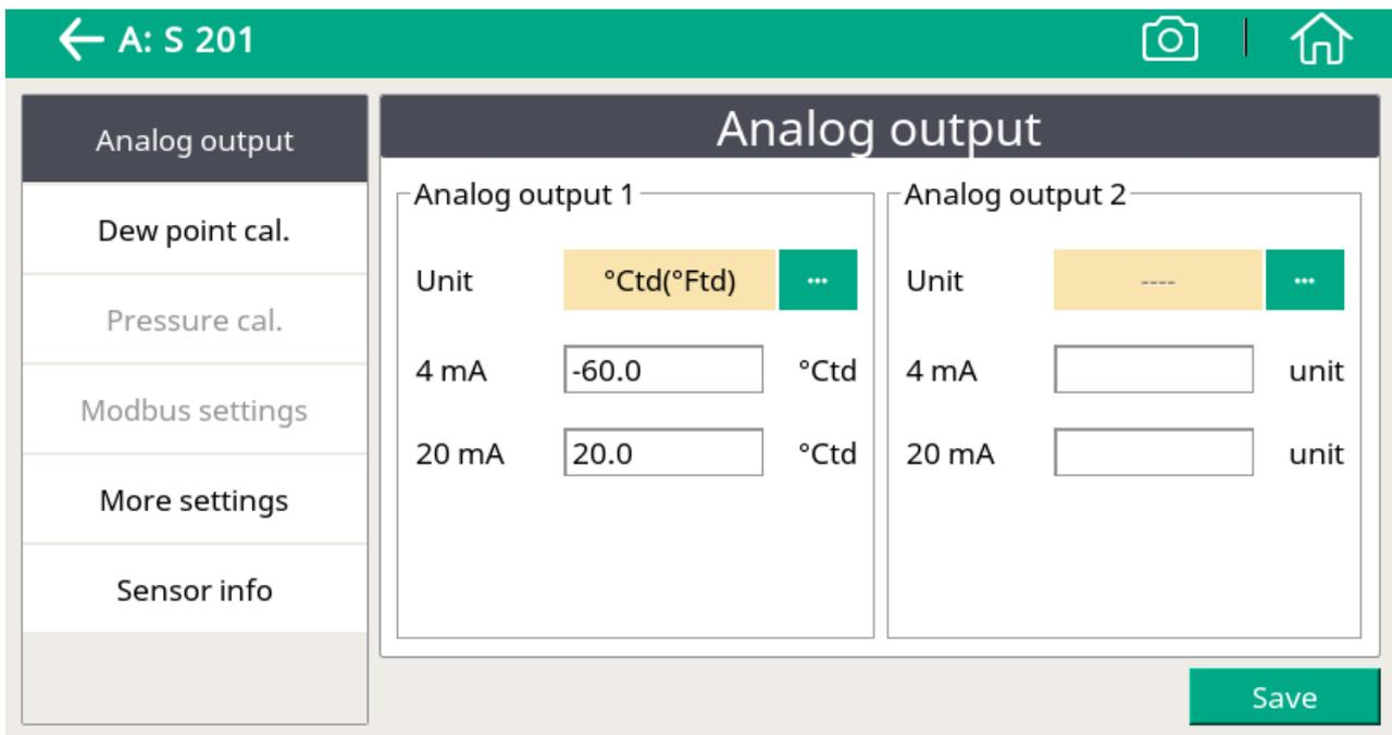
**Analog output** Select the physical moisture unit and set scaling for the analog output:
