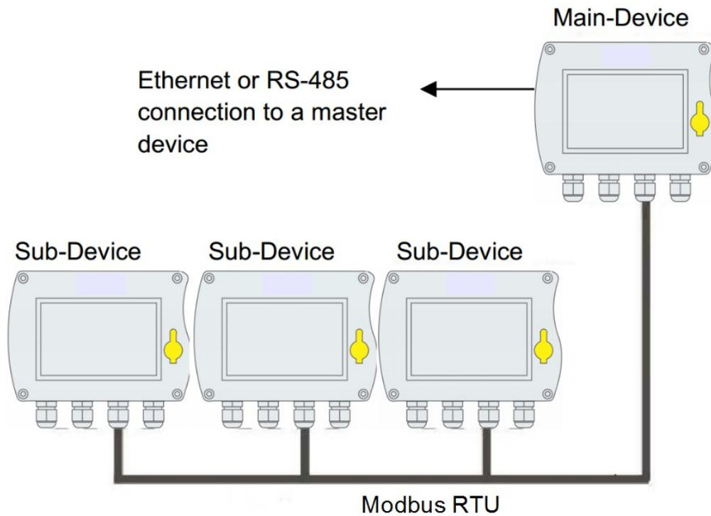
The above picture shows that S330/S331 (Sub-Device) - or any other device that has a Modbus/RTU interface can be connected to a Modbus-Master (Main-Device) through Modbus/RTU.
