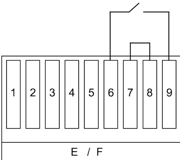
**F.** Connection of an active pulse signal from a flow meter or connection of a 24 VDC relay signal from a compressor for monitoring the run time of the compressor (For more details, see section [13.2](#).)
