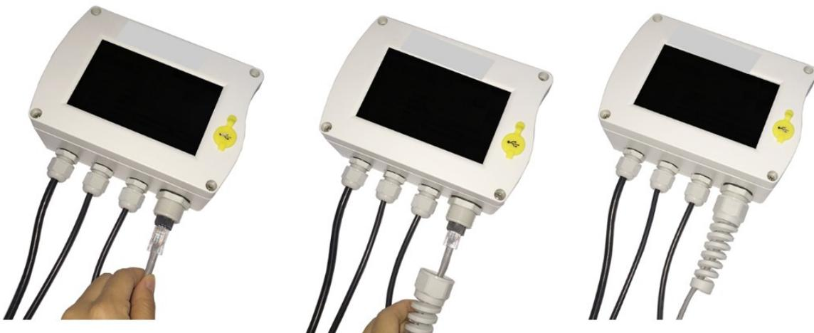
Connect Ethernet cable and mount bend protection sleeve
