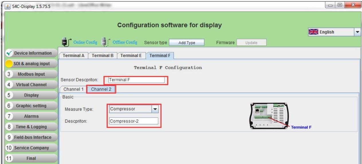
To reset the compressor run time, reset the Channel 2 on Terminal E or F. See the following figure for details.
