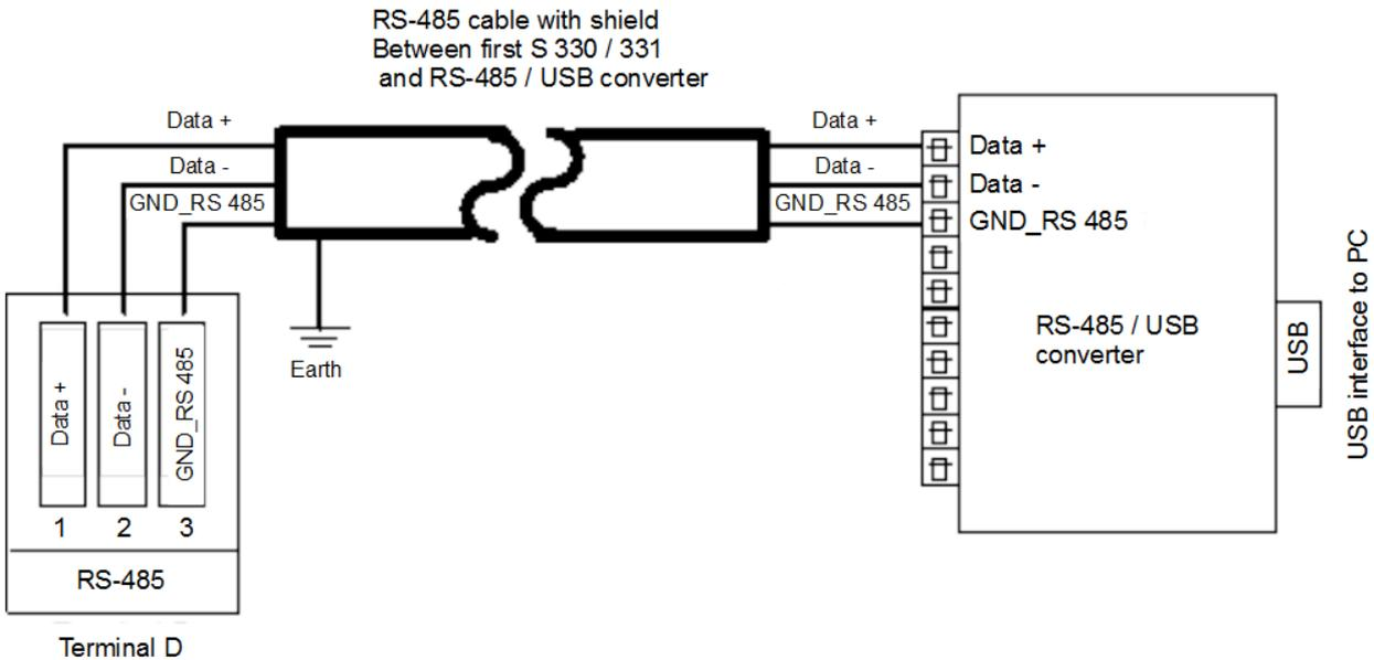
Through a RS-485 / USB converter the system is connected to a USB port of the office PC. RS485 network requires a termination resistor network. At both far ends of the devices, termination resistor must be turned on communication menu, all others S330/S331 remain off, Terminal resistor is software control in S330/S331. Please set it up correctly.
