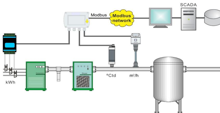
Modbus is a popular industry bus that can be used to connect several S330/S331 to a Modbus master. A PLC, a SCADA system, or a S330/S331 Master can work as the Modbus master.
