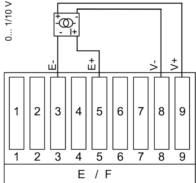
**E.** Connection of an isolated pulse input from a flow meter or connection of a relay signal from a compressor for monitoring the run time of the compressor (For more details, see section [13.2](#).)
