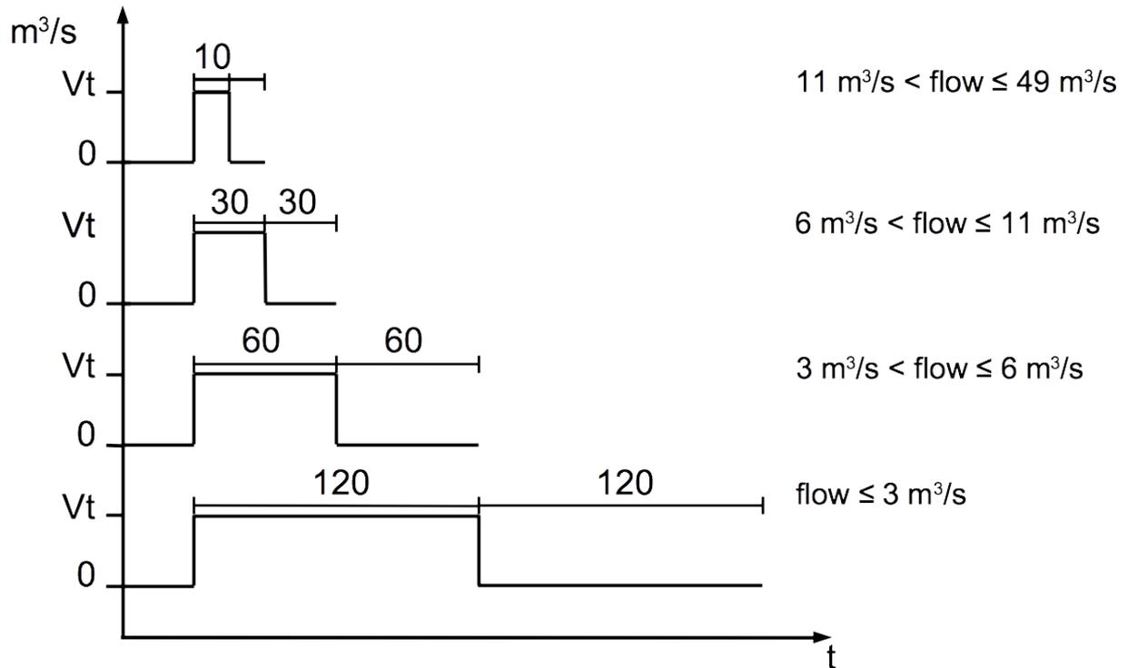
If the flow rate is too high, the S421 cannot output the pulses with default settings (one pulse per consumption unit). In this case, the pulse can be set by our service software or a connected display to 1 pulse per 10 consumption units or 1 pulse per 100 consumption units. For example, if set to 1 pulse per 10 m<sup>3</sup>, the sensor sends one pulse each 10 m<sup>3</sup>. Example (1 pulse per 10 m<sup>3</sup>):
