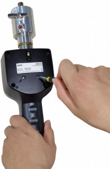
1. Open the two screws at the back of the instrument.
