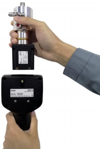
2. Pull the sensor unit together with the measuring chamber out of the main unit.
