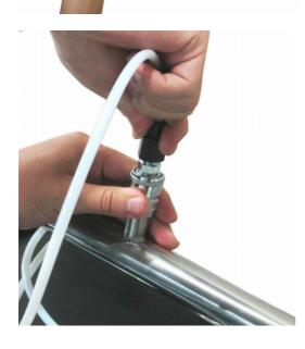
3. Connect the quick coupling at the other end of the teflon hose to the process.
