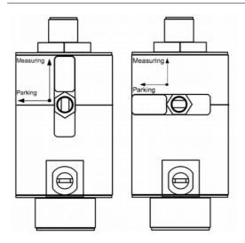
5. Turn the handle on the chamber to the "Measuring" position.
