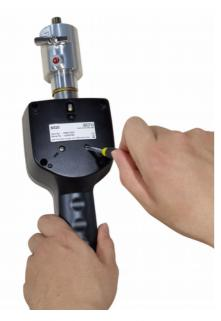
1. Open the two screws at the back of the instrument.
