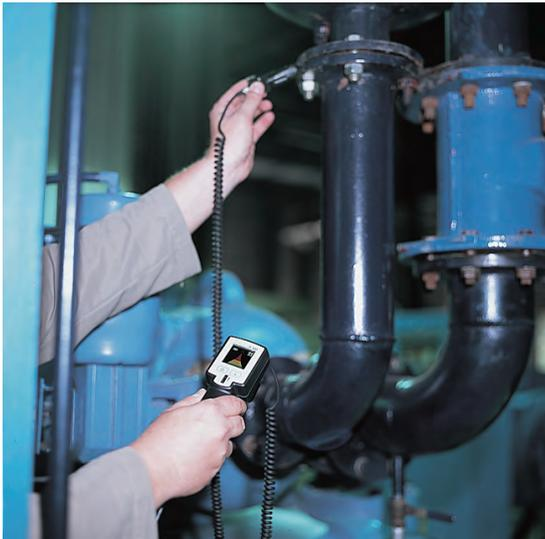
Leak detection with focus tube
