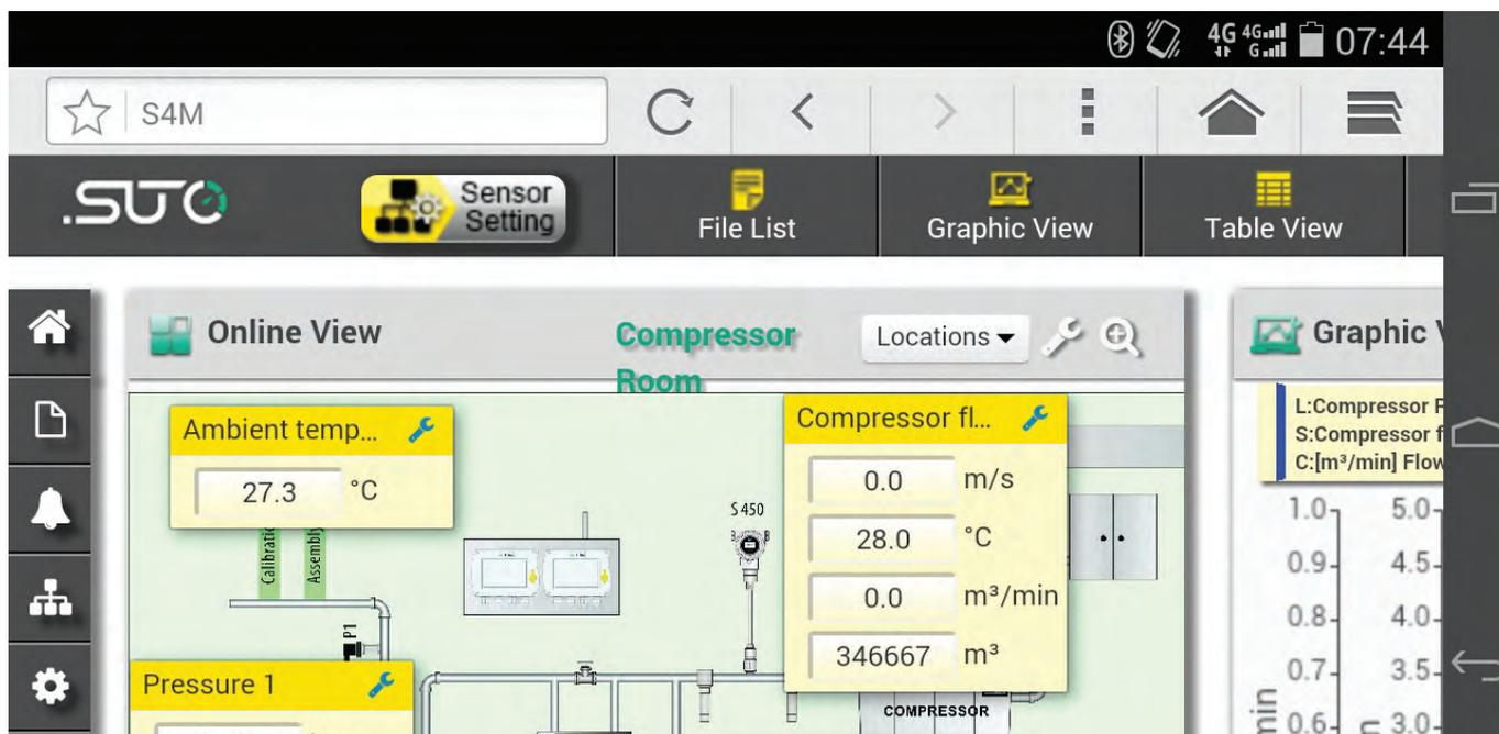
Above is an example show monitoring of a typical compressed air system with all relevant online parameters displayed on the screen.
