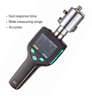
With the S 505 SUTO has combined next generation measurement technology with modern user interface design. The experienced user knows that dew point measurement also requires the measurement of line pressure (according to ISO 8573), since dew point is pressure dependent. With the S 505 the line pressure is measured in combination with the dew point, so the user can be confident that the calculation is accurate and free from human error.
