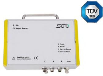
The S 120 oil vapor sensor monitors the oil content of compressed air and gases permanently or for spot checks when used as portable unit in conjunction with S 551. For best accuracy and long term stability, the S 120 sensor applies an automatic calibration. Sensor contaminations and sensor life time are monitored and indicated to the user. An 'over range' detection removes the sampling air from the sensor to protect it against contamination.
