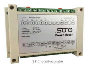
The S 110 Power Meters are designed for easy installation and high accuracy. They measure the actual power consumption in kW and accumulate the Energy consumption in kWh of a 3-phase load. The S 110 can measure other parameters such as current, voltage, cos phi etc. Hat rail, wall mountable and portable versions are available.
