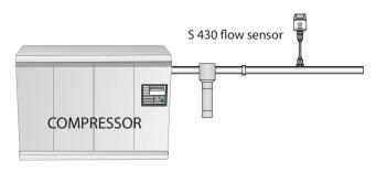
Compressor air delivery measurement and FAD calculation
