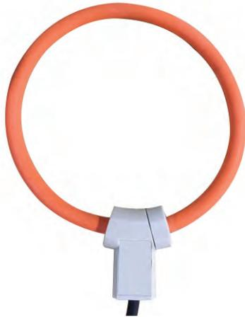
SUTO current clamp sensor is an AC RMS current sensor composed of a flexible active part (Rogowski coil model) connected to a compact digital converter, capable of measuring the current carried on a power conductor up to a value of 3000 A AC.
