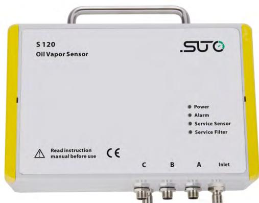
The S 120 oil vapor sensor monitors the oil content of compressed air and gases permanently or for spot checks when used as portable unit in conjunction with S 551. For best accuracy and long term stability, the S 120 sensor applies an automatic calibration. Sensor contaminations and sensor life time are monitored and indicated to the user. An 'over range' detection removes the sampling air from the sensor to protect it against contamination.
