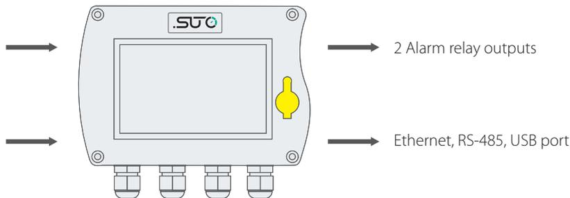
SUTO sensors are equipped with SDI and / or Modbus interface
