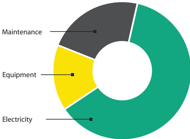
When looking at the overall costs of a typical compressed air system, the biggest costs are caused by the electrical power consumption but not by the investment or maintenance of the system.
