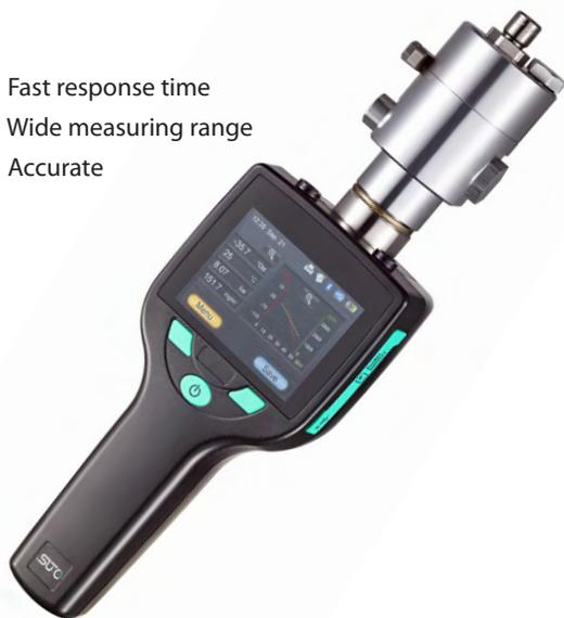
With the S 505 SUTO has combined next generation measurement technology with modern user interface design. The experienced user knows that dew point measurement also requires the measurement of line pressure (according to ISO 8573), since dew point is pressure dependent. With the S 505 the line pressure is measured in combination with the dew point, so the user can be confident that the calculation is accurate and free from human error.
