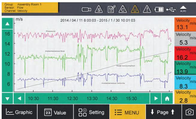
The S 330/331 comes with a high resolution 5" colour touch screen interface making the operation as simple as possible.
