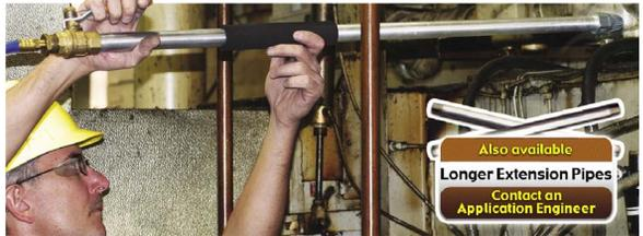
The 3' extension on the Model 1215-3 Super Blast Safety Air Gun helps an operator provide maximum blow off force to remote, tight or difficult to access areas.
