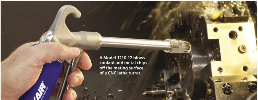
A Model 1210-12 blows coolant and metal chips off the mating surface of a CNC lathe turret.
