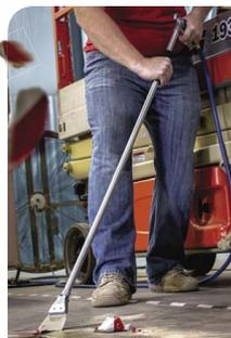
The Model 1244-36 scrapes and blows old tape off a concrete floor.
