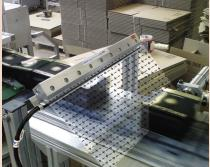
The Problem: A manufacturer of perfumes and fragrances had a problem with the packaging of their fine perfumes. The conveyor belt used to transport the boxes to the cellophane sealer rubbed against the box surface and induced a sizable static electricity charge on it that made it a "dust magnet". The cardboard dust and particulates
