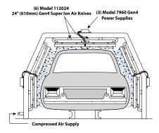
EXAIR's EFC (*shown on page 7*) is an electronic flow control for compressed air. It can sense when there is no car present and will automatically turn off the compressed air until the next car is moved into position. It is a perfect addition to this type of application.
