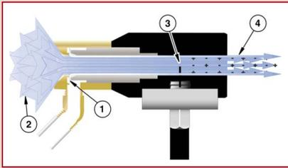
The Gen4 Ion Air Gun incorporates a High Velocity Air Jet and electrically energized emitter point. A small amount of compressed air is injected into the air jet (1) inducing high volume flow of surrounding air (2) to pass through it.
