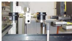
(2) Model 120022 2" (51mm) Super Air Amplifiers dry small parts as they move down along a parts conveyor.
