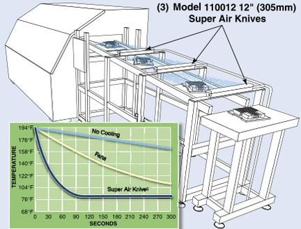
**Comment:** The laminar airflow of the Super Air Knives was the key to success in this application. Fan cooling could only provide random spikes of air at moderate velocities. **The uniform sheet of air from the Super Air Knife quietly swept the heat away within the first 2' (610mm) of the conveyor.** Low air consumption and the compact size of the Super Air Knife were an added bonus.
