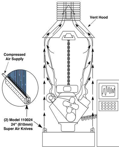
**The Problem:** The last step in an engine assembly process is “burn-in” on a test stand. Each engine is connected to a dynamometer and run for a period of one to five minutes. Residual machining oil on the head produced smoke during the test, and the vent hood at the top of the stand had insufficient capacity to contain it.
