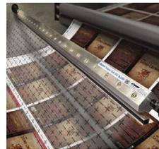
The Model 112048 48" (1219mm) Gen4 Super Ion Air Knife neutralizes the static electricity and cleans the surface of the paper.
