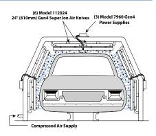
EXAIR's EFC (shown on page 7) is an electronic flow control for compressed air. It can sense when there is no car present and will automatically turn off the compressed air until the next car is moved into position. It is a perfect addition to this type of application.
