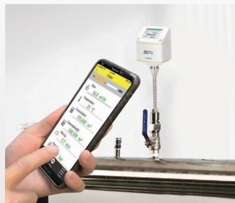
Sensor configuration through wireless connection
