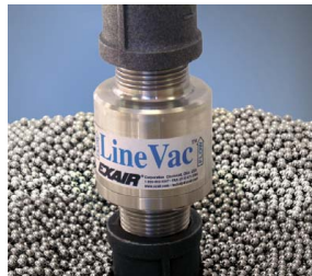
A drawer slide manufacturer conveys ball bearings with the Model 141125 1-1/4 NPT Stainless Steel Threaded Line Vac to an assembly station.
