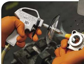
The Model 1699-CS removes chips and coolant from a machined part.
