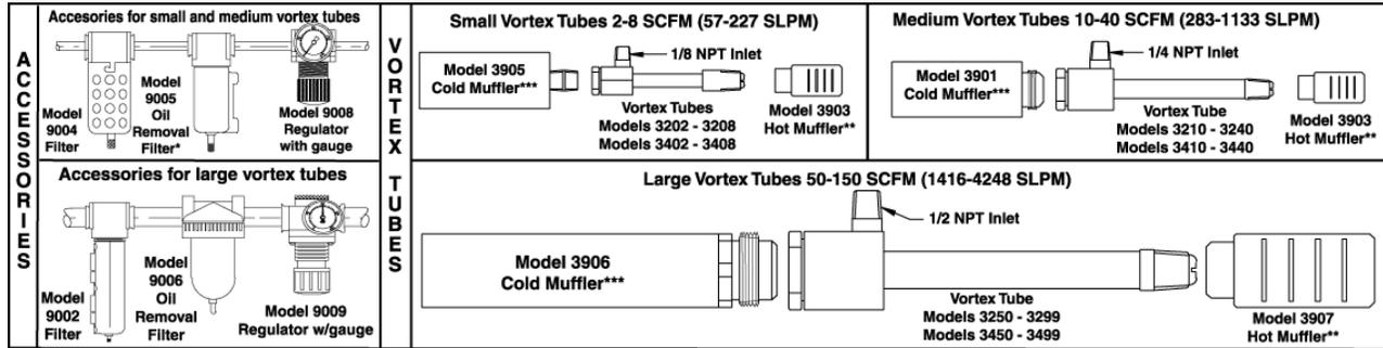
\*Use Model 9006 Oil Removal Filter for Vortex Tubes larger than 30 SCFM (860 SLPM)
